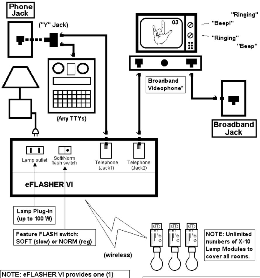
NOTE: eFLASHER VI provides one (1) flash for each telephone ring and double-flashes (2) for each Broadband ring.
