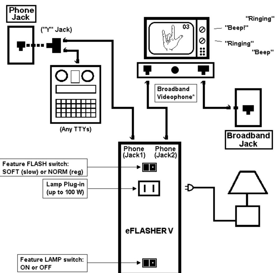
NOTE: eFLASHER V provides one (1) flash for each telephone ring and double-flashes (2) for each Broadband ring.
