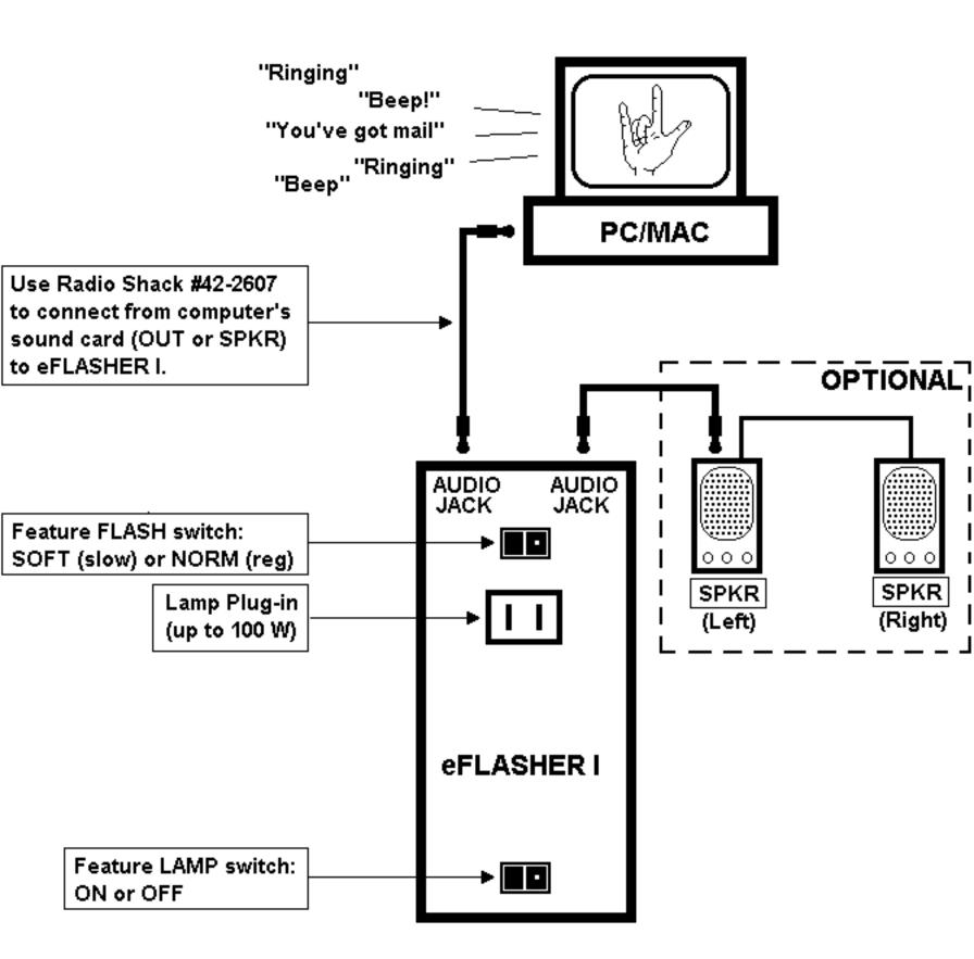
NOTE: eFLASHER I provides three (3) flashes for each computer sound or call signal received. Must use a special .WAV file to operate it which it can be download from manufacturer's website:
